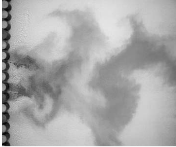
FIGURE 2. Dye visualization obtained for a grid with S=80\% , D=0.125 m, h=0.045 m, U=0.05 m s -1 . The area covered is 2.7 m \times 2.2 m with the water flowing from left to right. Dye is injected at two locations 0.47 m apart.
